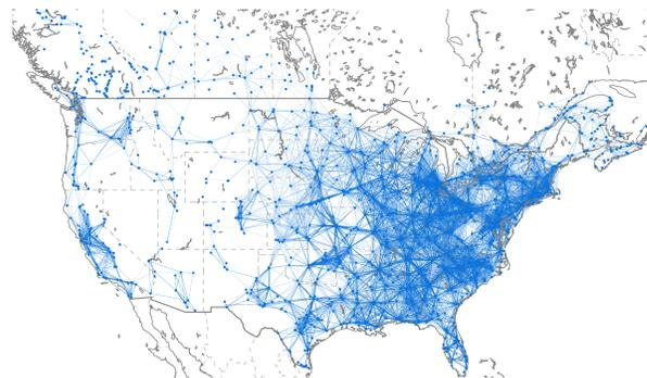
Fig. 1. Interference graph visualizing the constraint data (2990 stations; 2575466 channel-specific interference constraints).
